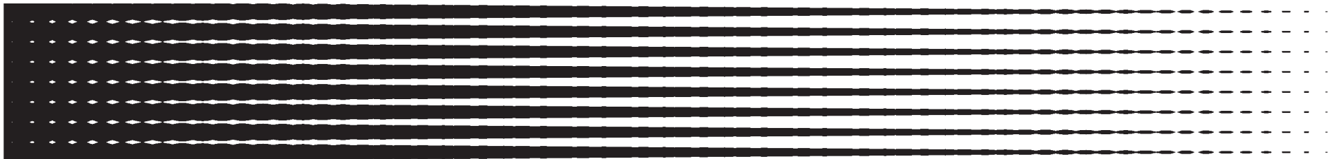
Figure 66: Megadot dot shape for cyan, magenta and yellow (enlarged).
