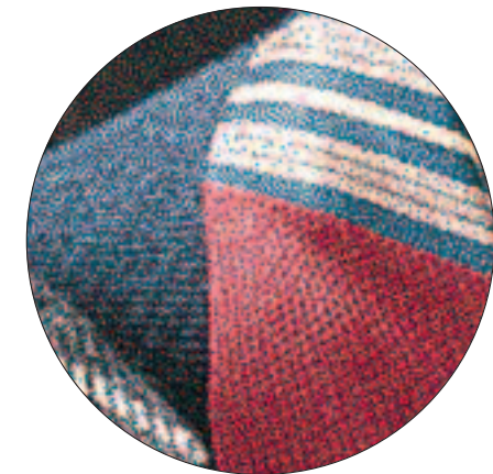
Figure 60: Enlarged section from the Prinect Stochastic Screening II medium screen.
