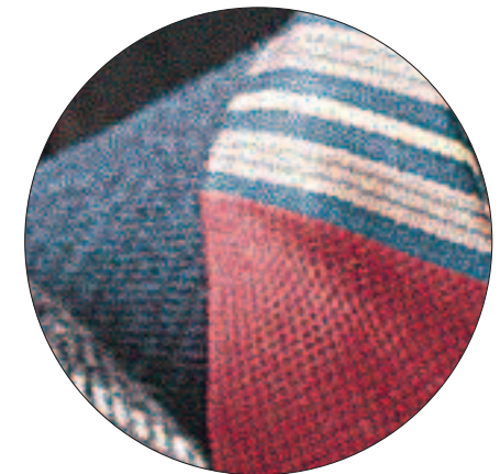
Figure 58: Enlarged section from the Prinect Stochastic Screening II fine screen.
