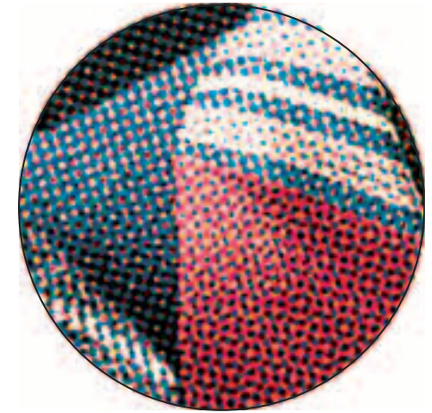
Figure 54: Enlarged section from the AM screen (IS Classic).
