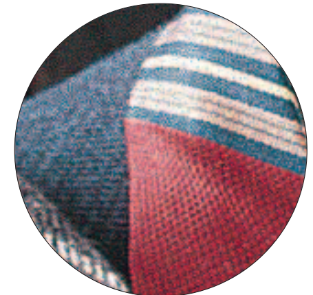
Figure 55: Enlarged section from the FM screen (Prinect Stochastic II fine).
